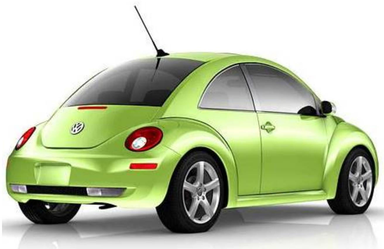
But there are a few things one should know before starting with a road test. Volkswagen has perfected the art of platform sharing and deep under the stunning shell of the bug lies a VW Golf (ditto with other VW Group models like the Skoda Octavia, Audi TT and so on). That means the new car features a front-engine, front-wheel drive lay out instead of the rear-engine, rear-wheel drive lay out of the original. No more 'bonnet' jokes alright?
